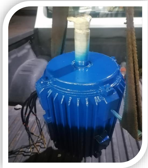
Motor de 7.5 kw, Voltaje 480 VAC, 12.1 AMP, 1750 RPM, 60 HZ
